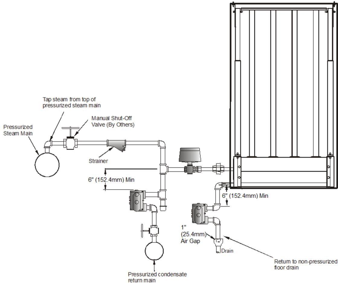
**Note: The SAM-e header functions as a steam separator, therefore an external steam separator is not required.**
