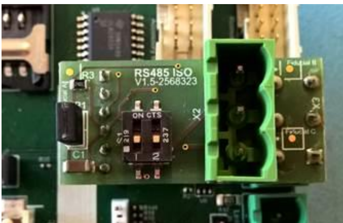
Fig. 4: Mounting the "Isolation Module" option
